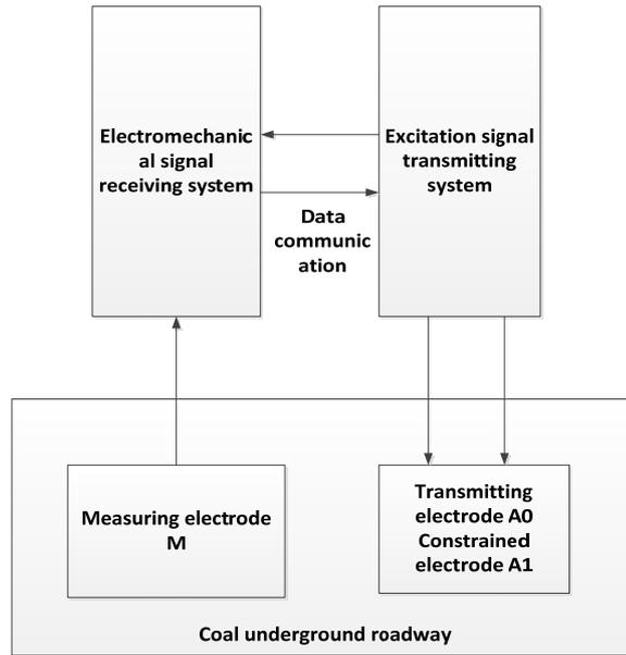
**Figure 1 Dual-frequency IP detection system**
