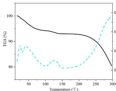
Figure 2. TGA and DTG thermal curves
