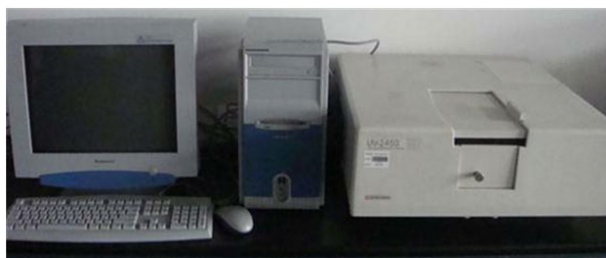
Fig. 2. An instrument for the determination of Cr 6+
