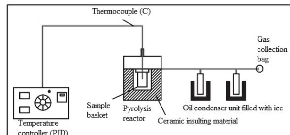
Fig. 2. The pyrolysis system.
