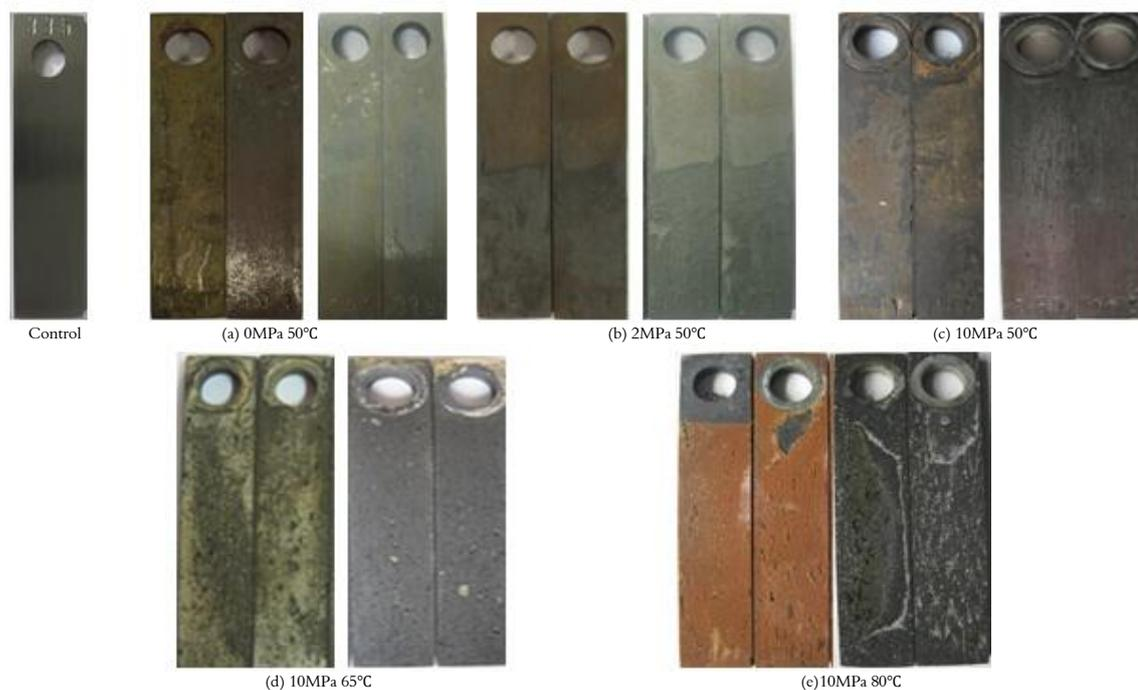
**Fig. 2.** Corrosion product film morphology of corroded samples at difference CO<sub>2</sub> pressures and temperatures
