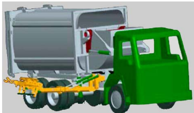
Figure 1 Virtual prototype model of side-mounted garbage truck manipulator
