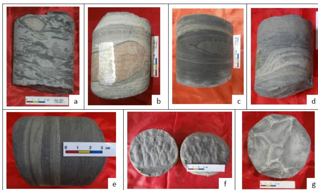
a. Well Z46, 695.08m, shale swarf, “mud-coated” structure; b. Z46 well, 751.4m, “mud-coated “ structure; c. Well N24, 1500.61m, wrap bundling; d. Well Z55, 1229.30m, sand pillow structure; e. Well Z55, 1238.00m, Bouma sequence DE; f. Well N38, 1733.81m, slot mode; G. Well N20, 1654.84m, heavy mode
